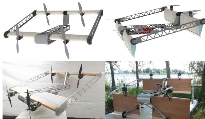
Figure 4-8: Rendering (top) and first prototype of the TiltOne (bottom)
